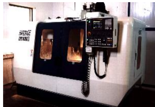
数控镗铣加工中心 N/C BORING AND MILLING MACHINING CENTER
